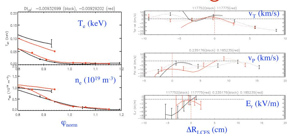
• ERD measured profiles of NBI and RF parameters are within experimental errors prior to H-mode.
