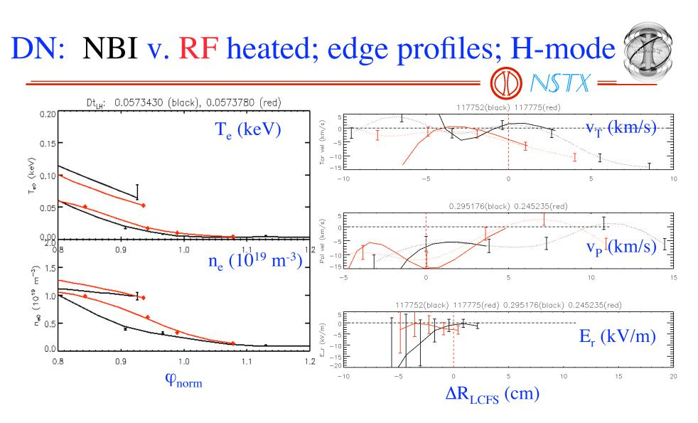
• During H-mode less agreement between edge ion parameters, especially  $v_T$
