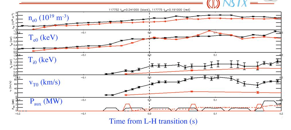
T<sub>i</sub>, v<sub>T</sub> measurements made using CHERS
