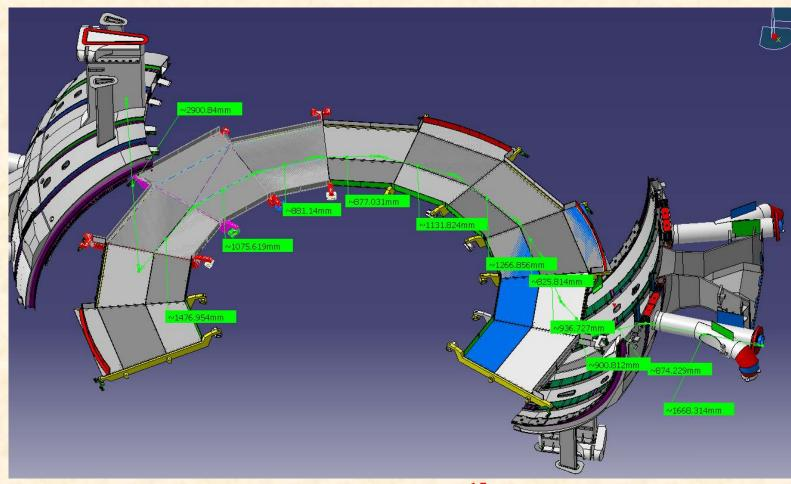
Estimated cable length from Oct outer limiter guide tube to top of outer vessel at Oct  $5 = \frac{-15m}{10}$  However, some extra might need to be added to be safe. This does not include the length required ex-vessel to the power supply etc.
