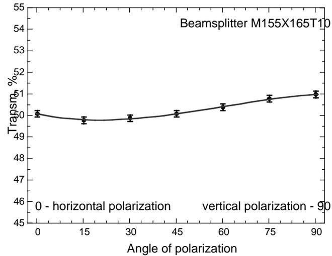
Dependence of transmissivity vs. Angle of polarization.
