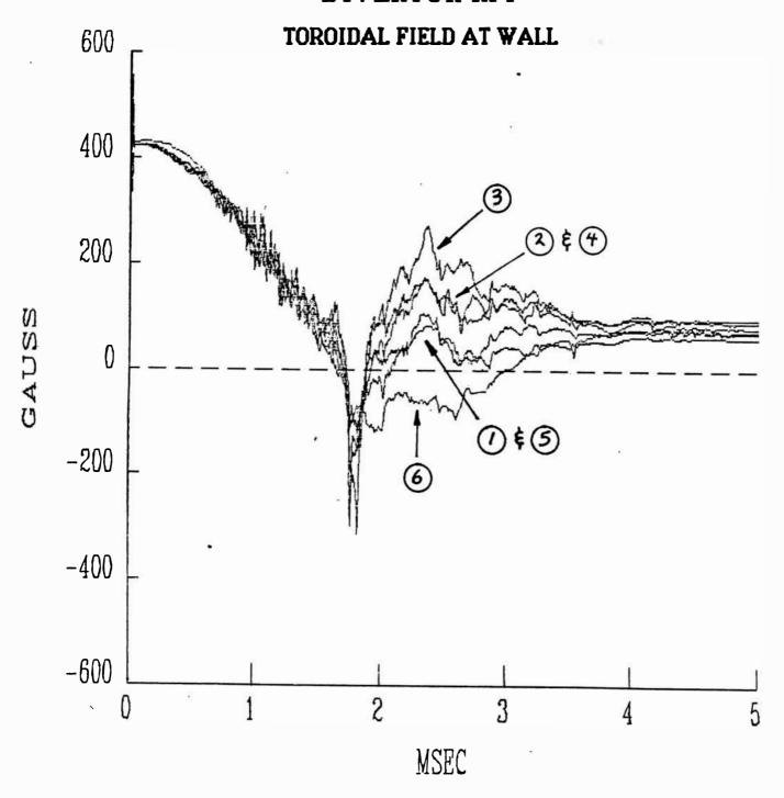
This figure illustrates the poloidal asymmetry in the magnetic field at the edge of the plasma. The five probe signals fit well to an m=1 distribution.
