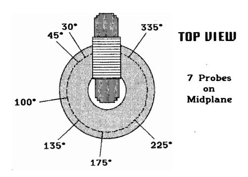
Seven small magnetic probes were separated toroidally to check toroidal symmetry. The coils were located near the vacuum vessel wall on the midplane.
