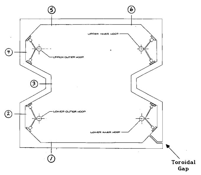
Six small magnetic probes were separated poloidally to check poloidal symmetry. The coils are located near the wall at the 225° toroidal azimuth. The values of  $RB_{\emptyset}/R_3$ , where  $R_3$  is the major radius at which coil 3 is located, are plotted below.
