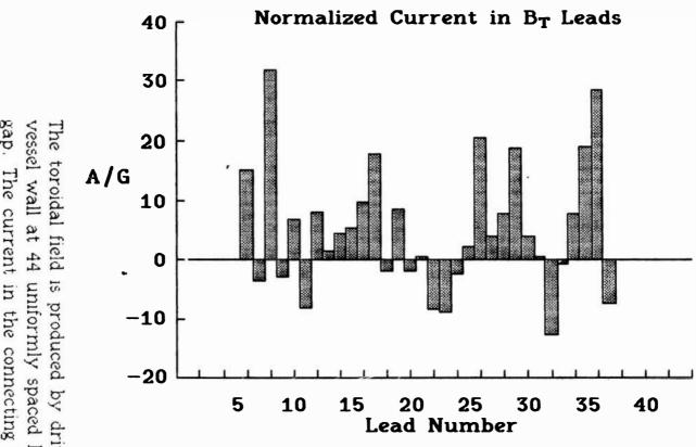
for both the plasma and vacuum cases. The current in produced by driving the aluminum vacuum the connecting leads is highly non-uniform locations around the toroidal
