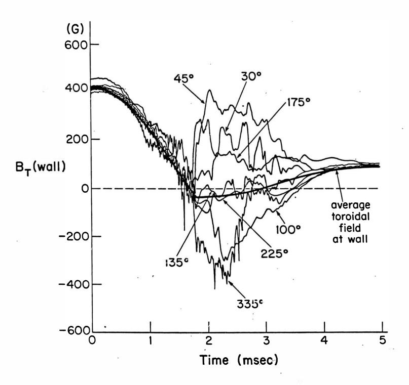
This figure illustrates the toroidal asymmetry in the magnetic field at the edge of the plasma. Similar behavior is observed at the center of the plasma when the probes are inserted in that region. 8
