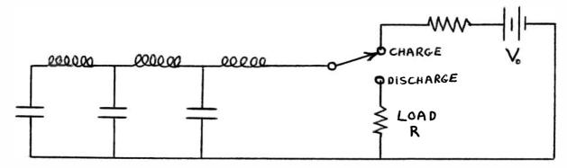
If the line is matched to the load (Z = R), the voltage developed across R is  $V_0/2$  and has a duration of 2T. For Z  $\neq$  R, a reflected wave is produced, the initial voltage at the load is
