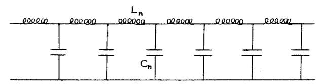
An ''ideal'' transmission line has an infinite number of such LC networks, so that  $L_n$  and  $C_n \to 0$ . The fundamental equations for a transmission line are
