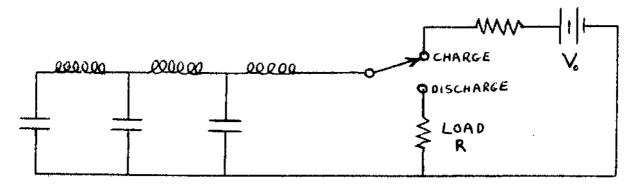
If the line is matched to the load (Z = R), the voltage developed across R is  $V_0/2$  and has a duration of 2T. For Z  $\neq$  R, a reflected wave is produced, the initial voltage at the load is
