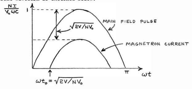
In practice, we usually want  $\omega t_0 < \frac{1}{2}$ , and so the turns ratio must be at least
