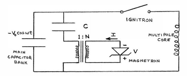
An extra capacitor (C) is added across the main bank in series with a transformer of turns ratio 1:N. Alternately, one of the existing capacitors could be used. The magnetron is represented by a zener diode of voltage V with current I. We ask how I
