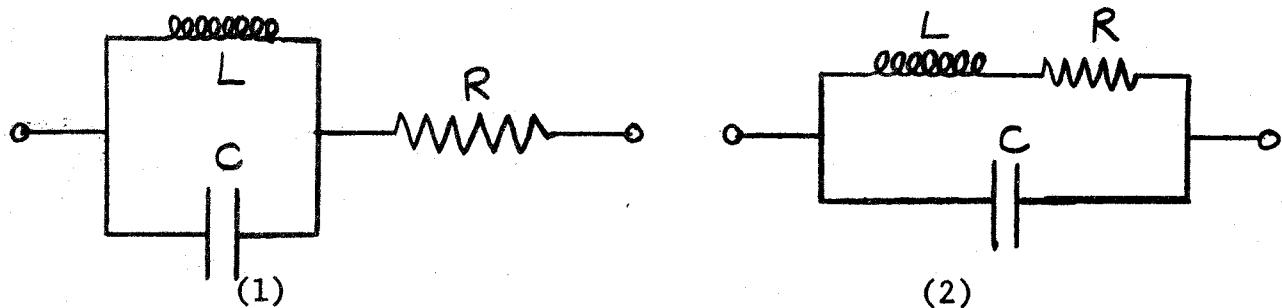
Since the capacitance is due to a displacement current across the sheath, circuit (2) would more nearly represent the physical
