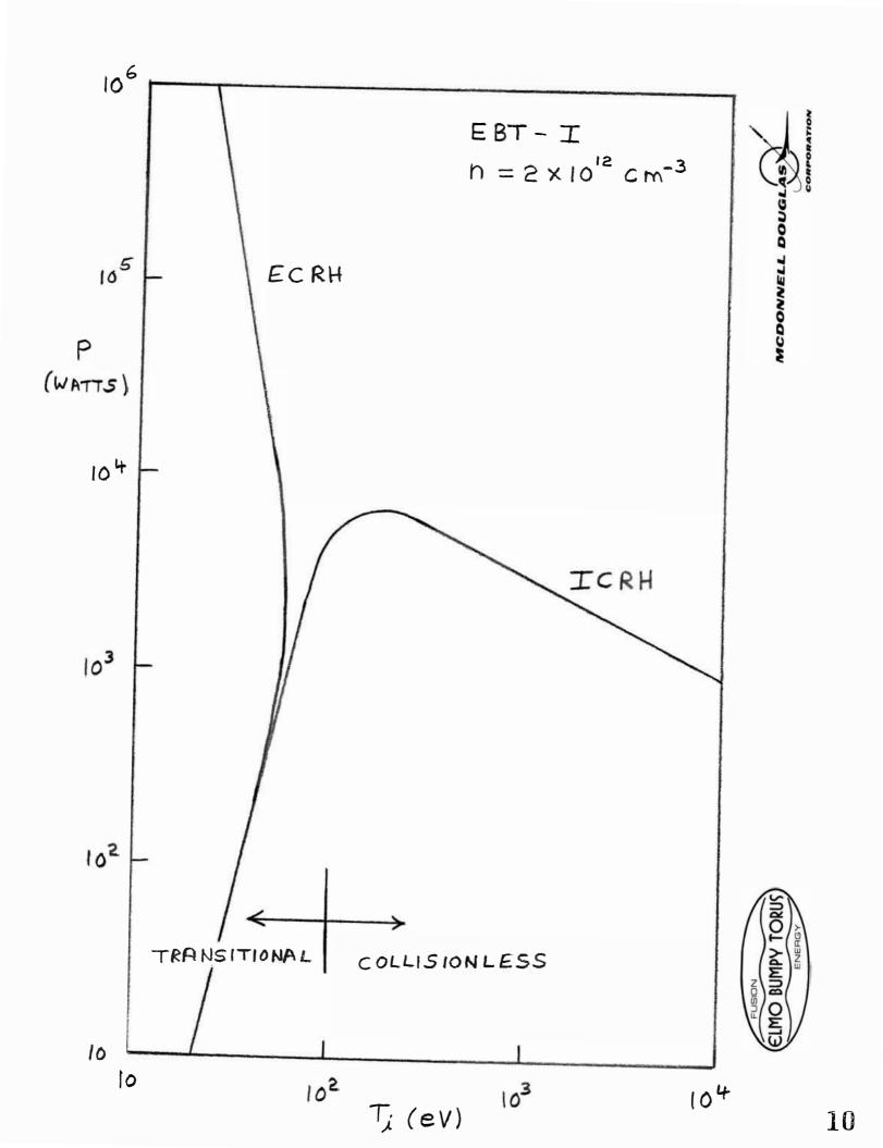
power. If the ECRH is removed and ICRH is used to sustain the bulk plasma, the electron temperature stays very close to the ion temperature in the collisional regime, but in the collisionless regime, the ratio  $F = T_e/T_i$  depends only on the aspect ratio:
