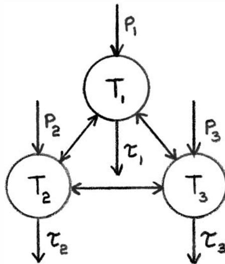
The input variables are the density of each specie (n), the input power to each specie (P), the energy confinement time for each specie ( $\tau$ ), and the atomic mass number (M) and charge (Z) of each specie. The output is the steady state temperature of each specie (T).
