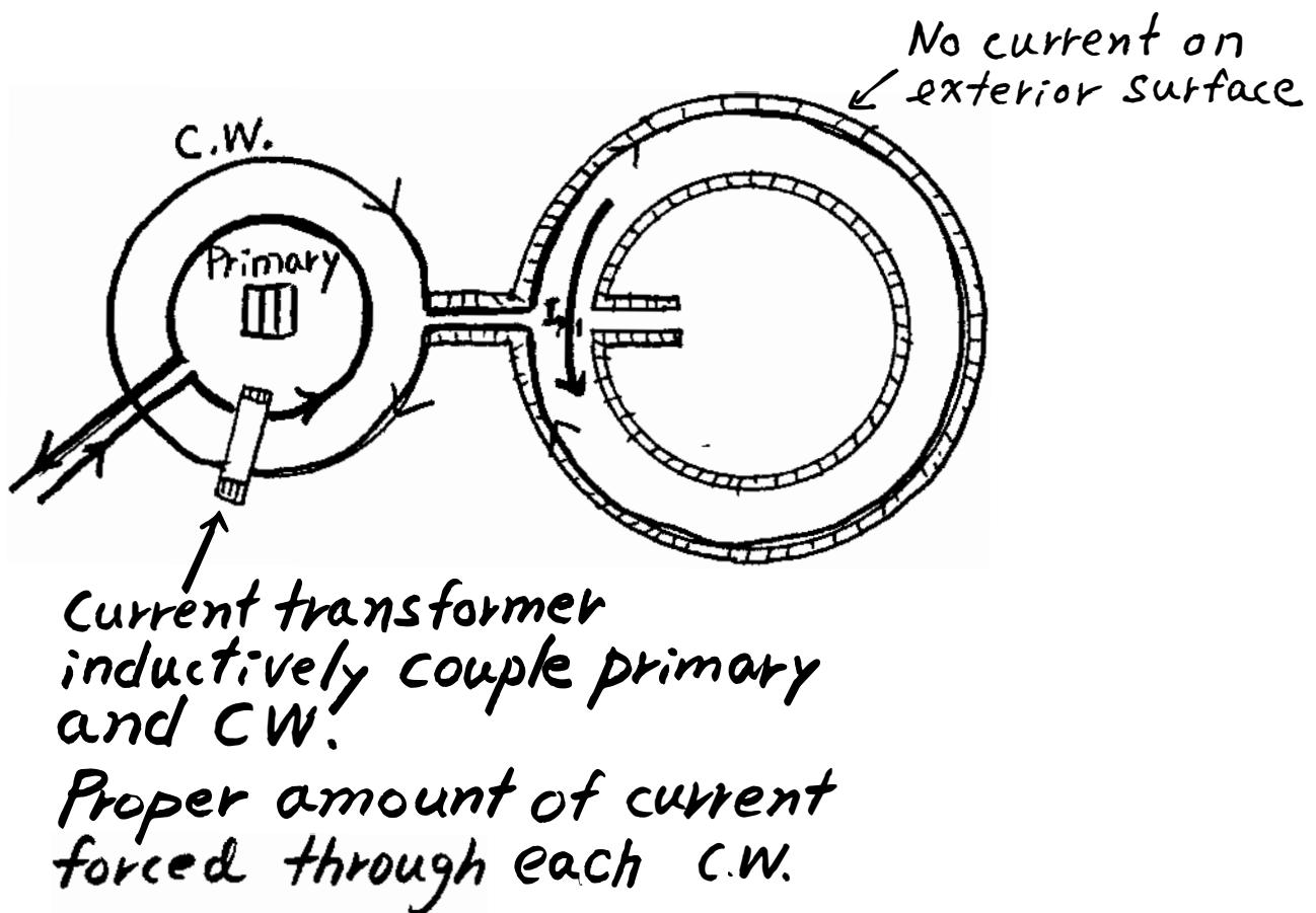
Proper placement of the C.W. system minimizes field-error.
