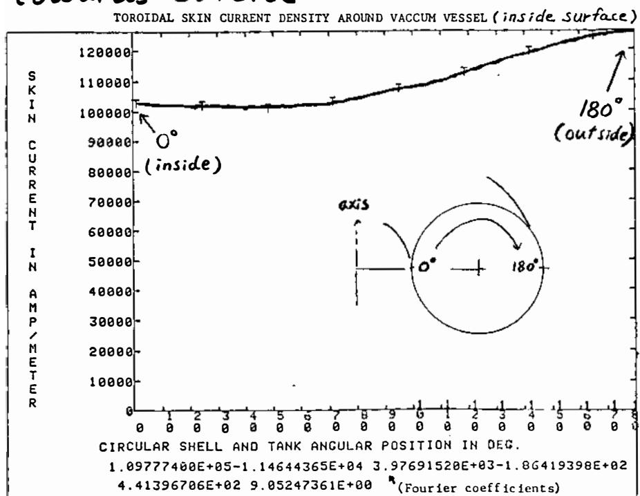
Without continuity windings, image current will flow on exterior surface of VCV
