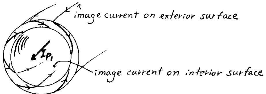
Continuity winding (C.W.) provide path for image current to go around the core.
