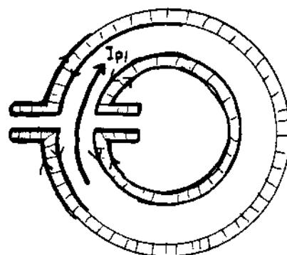
Flux plot exterior of VCV show  $\frac{J_{at\ 0^\circ}}{J_{at\ 180^\circ}} \geq 7$
