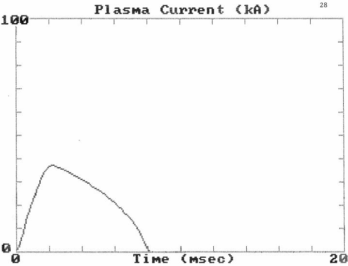
Fig. 12: Plasma current waveform for  $V_{\rm c}$  = 2500 volts and Z = 3 with the proposed new hoops.
