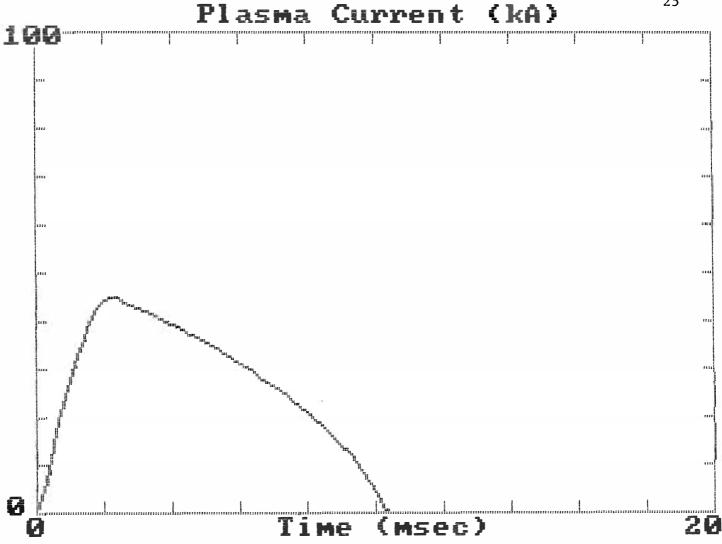
Fig. 9: Plasma current waveform for  $V_{\rm c}$  = 2500 volts and Z = 1 with the present hoops.
