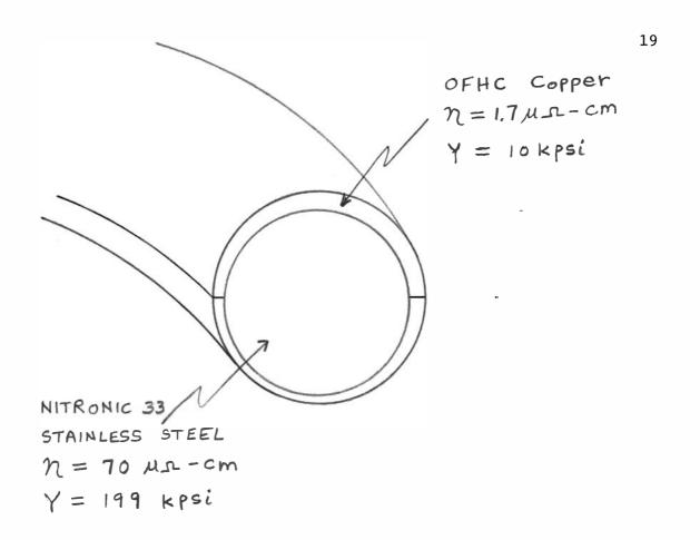
Fig. 8: Schematic illustration of proposed new Tokapole II hoops.
