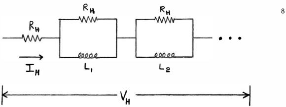
$R_{\rm H} = 8 \times 10^{-6}$  ohms (four CrCu hoops in parallel)
