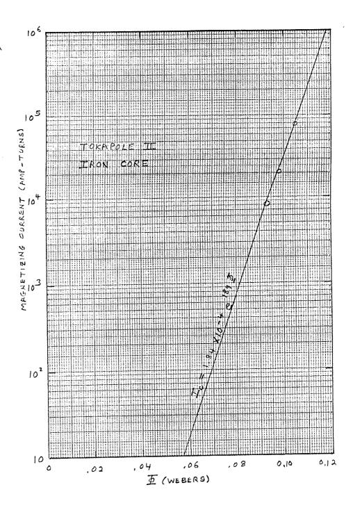
Fig. 4: Experimentally measured magnetization curve for the Tokapole II iron core.
